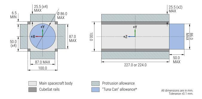
RAMI deployers accept two lengths of 2U CubeSats, the standard with 227.0mm, and the XL with 224.0mm.
