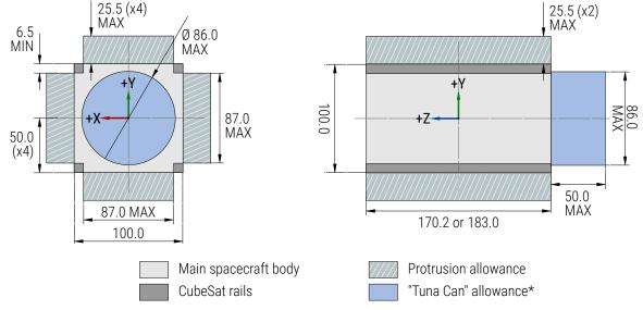
All dimensions are in mm. Tolerance ±0.1 mm.
