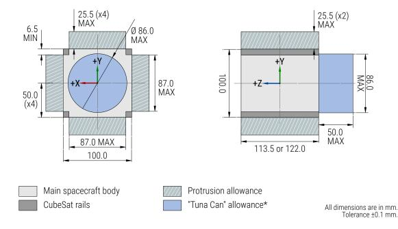
RAMI deployers accept two lengths of 1U CubeSats, the standard with 113.5mm, and the XL with 122mm. Customers can take advantage of the extra-room RAMI provides, including the 15mm of protrusions allowance in the dynamic envelope.
